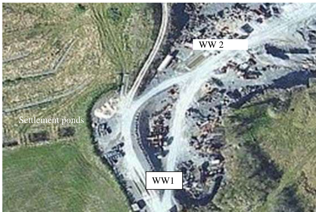
Plate 2.2 shows wheel wash locations (WW1/ WW2 located within the QMA Quarry Management Area. Aerial map also shows settlement pond location.
